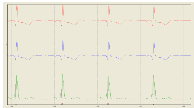
Figure 1. Three steps of the algorithm are shown: red is the input signal, blue is the filtered signal, and green is the absolute value of the first derivative.
